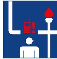
9. Ensure safe atmosphere in fire box before igniting the burners
