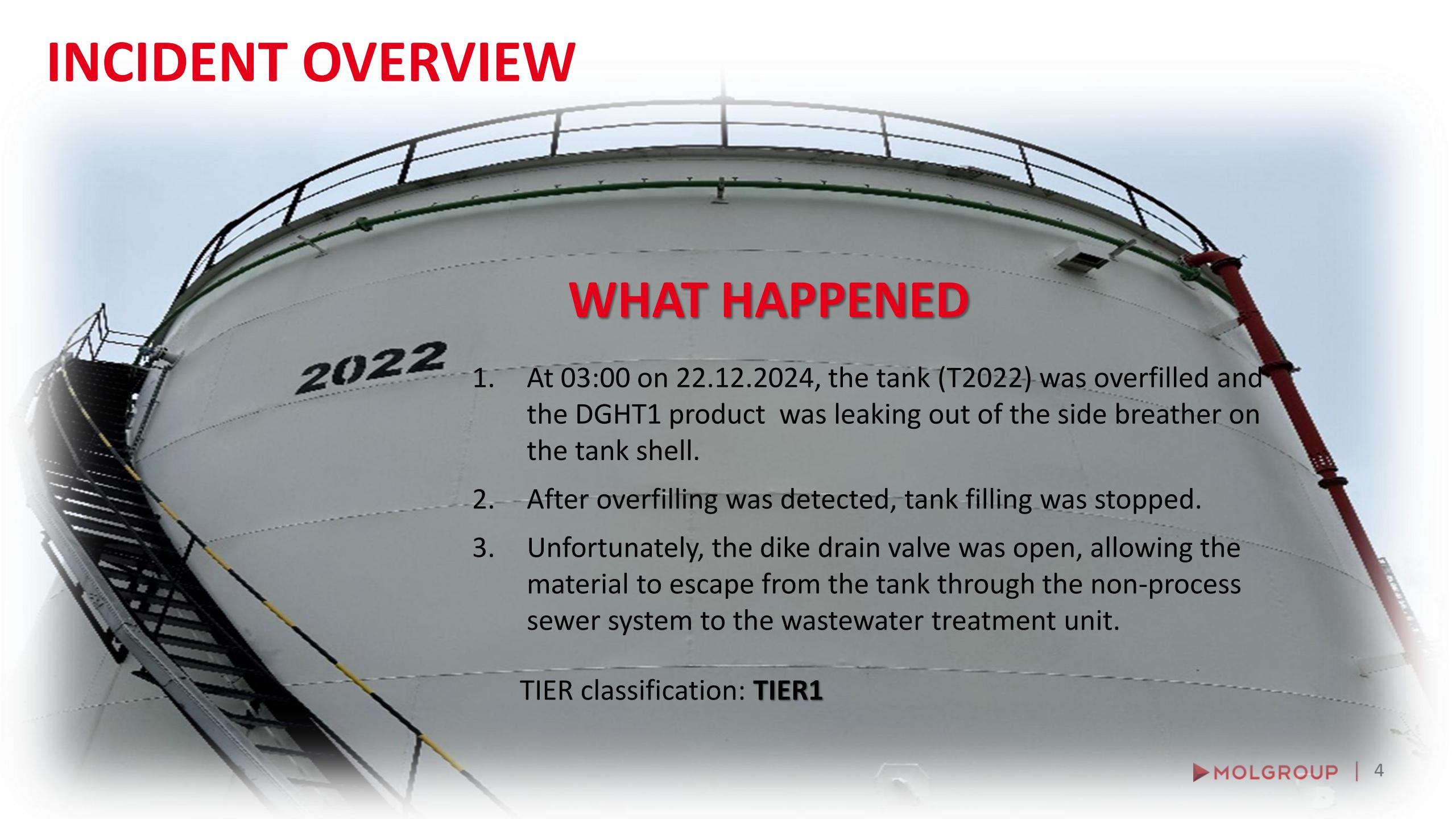
1. At 03:00 on 22.12.2024, the tank (T2022) was overfilled and the DGHT1 product was leaking out of the side breather on the tank shell.
