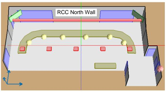
LEGEND: RED = Sound Sources (5 square air supply, 1 narrow air return and 1 indoor alarm) YELLOW = Receivers (from left to right: C1, C3, A1, A3, B1, B3 at 1.3 m above ground) GREEN = suspended LCD screens OLIVE = desks VIOLET = doors, wall LCD screens
