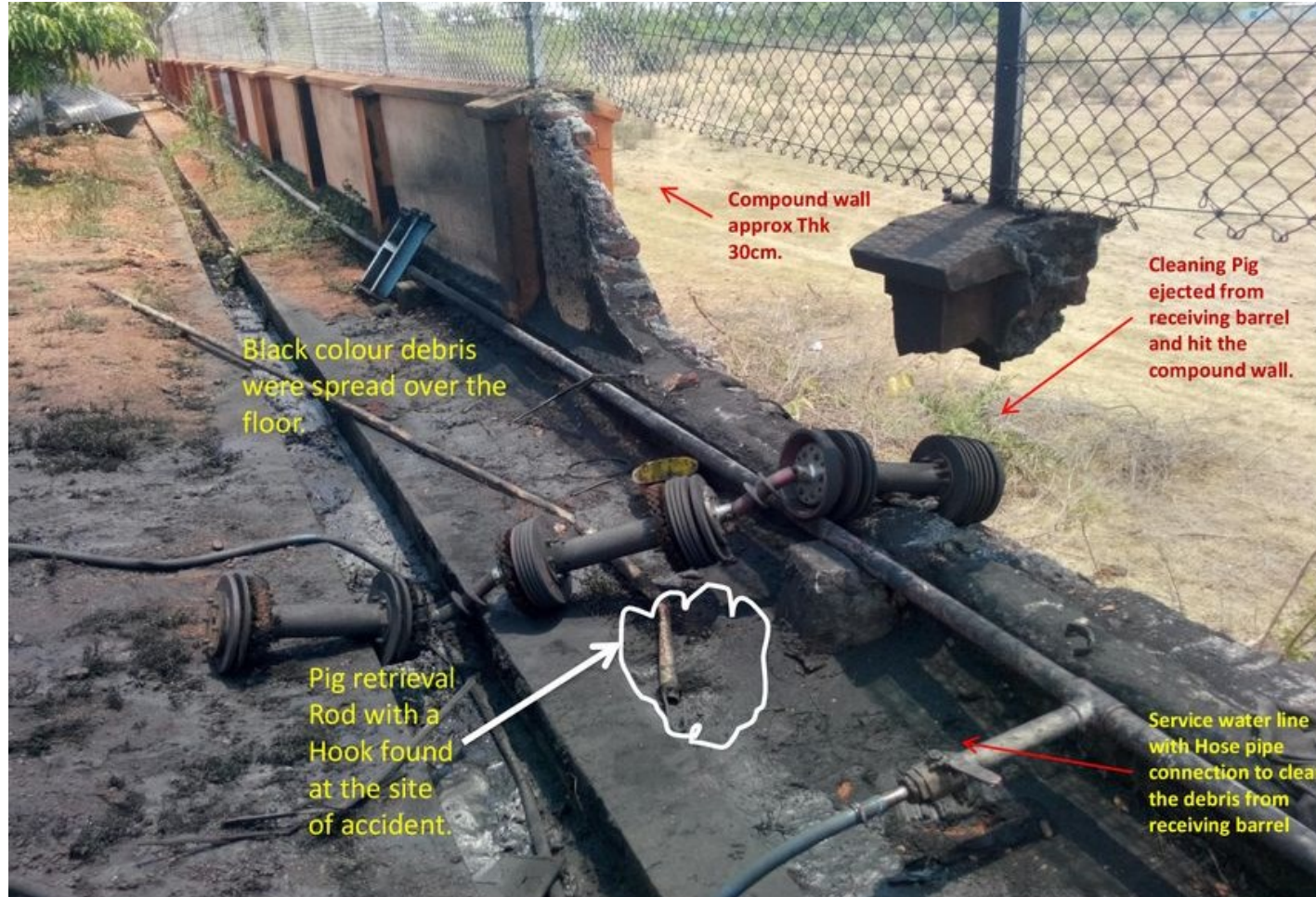
Pig Blew out of the Pig Receiver and hit the compound wall (about 9 meters from the Pig Receiver).
