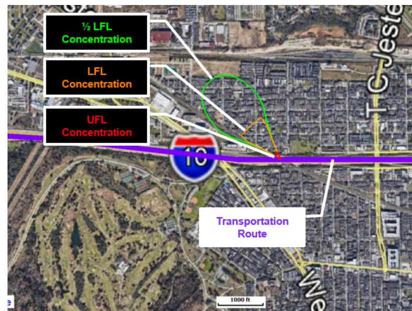
Flammable release – Flammability contours
