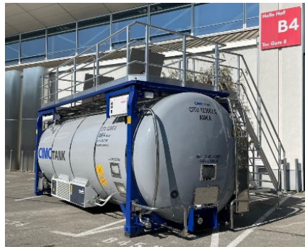
On-board chiller (reefer)
