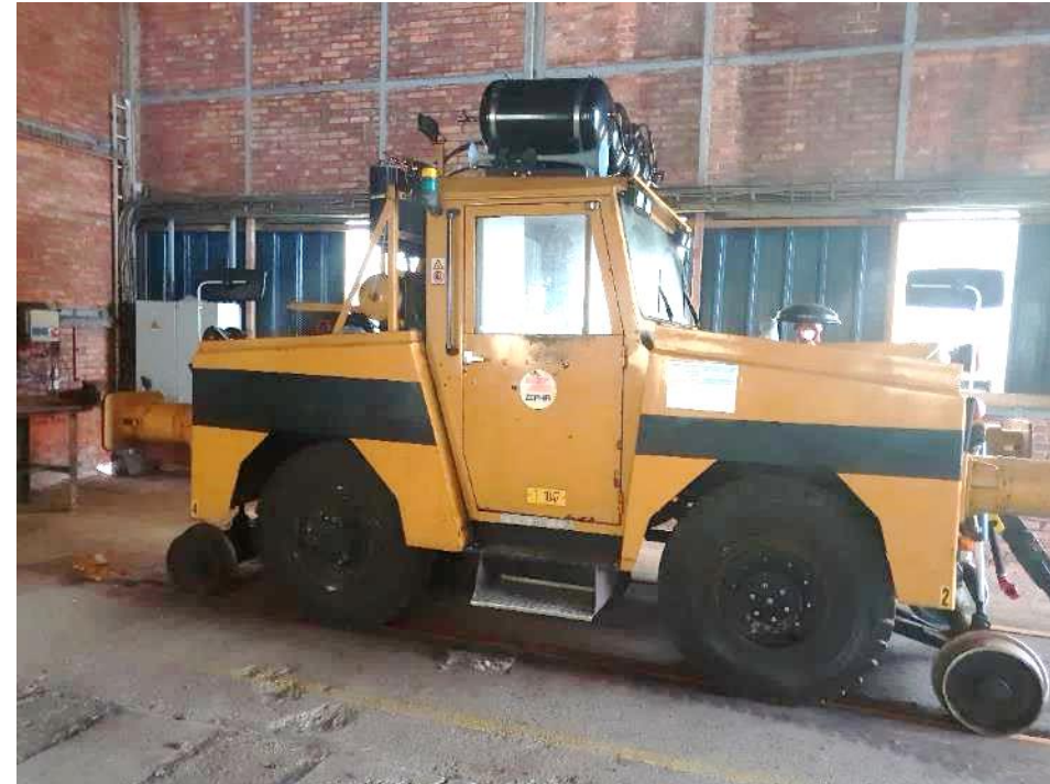
Light spare engine. Used during the incident. Only able to pull 4 loaded RCT instead of 8. Able to move 8 empty RCT at once
