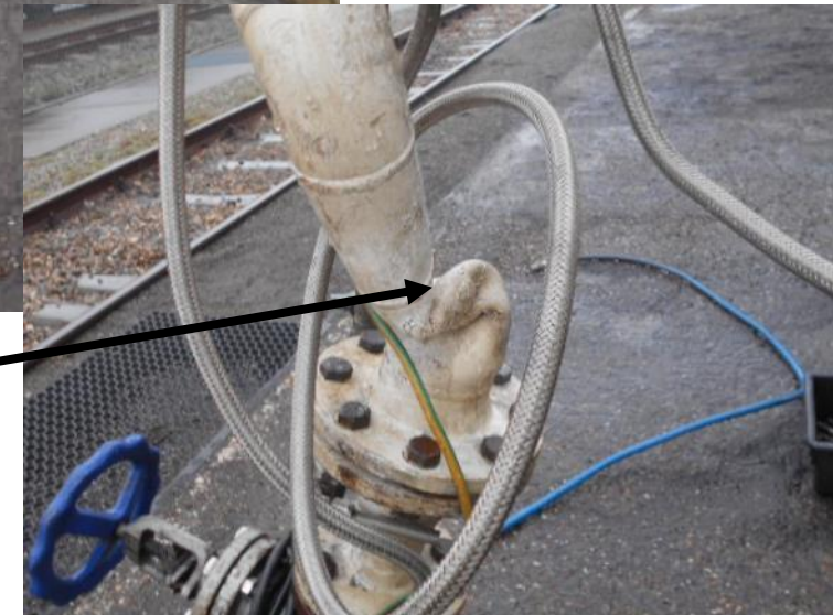
Loading arms gas and liquid phase severely damaged but not leaking
