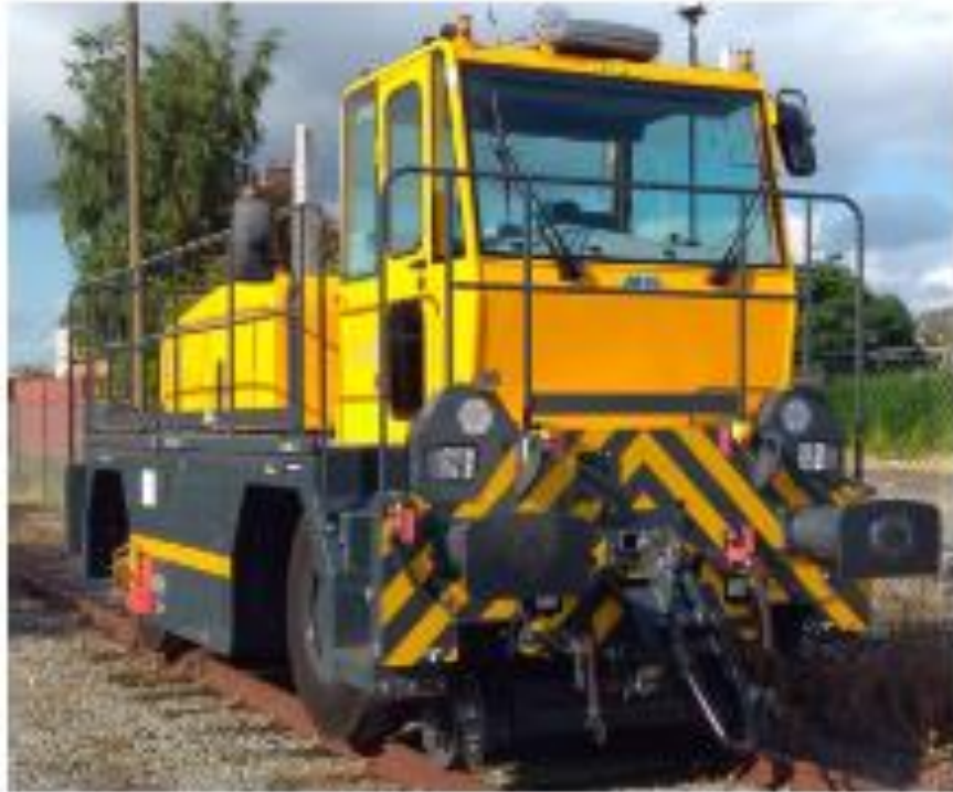
Heavy normal engine. In maintenance on the day of the incident. Able to pull 8 loaded RCT!
