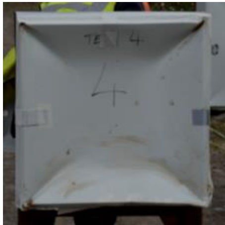
> 3 bar – Distortion of door and sides
