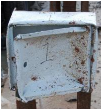
> 3 bar – Distortion of door and sides
