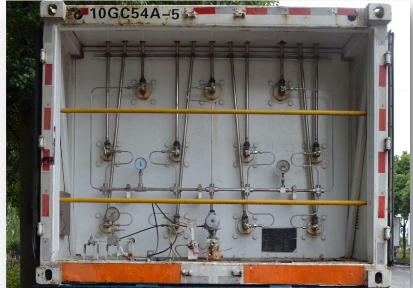
Picture 3: cylinder valves on the truck (left open the day of the event)
