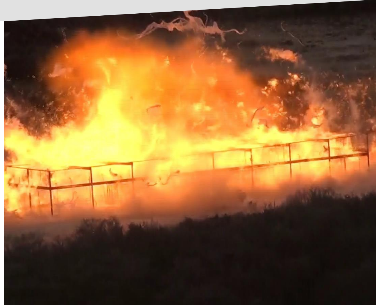
Large Cloud VCE Test at BakerRisk's BCTF
